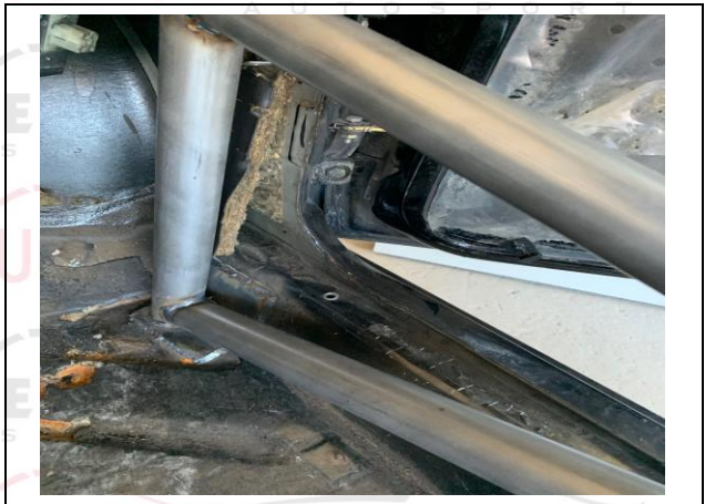
PHOTO 6 FRONT ROLLBAR TO FLOOR ATTACHMENT
