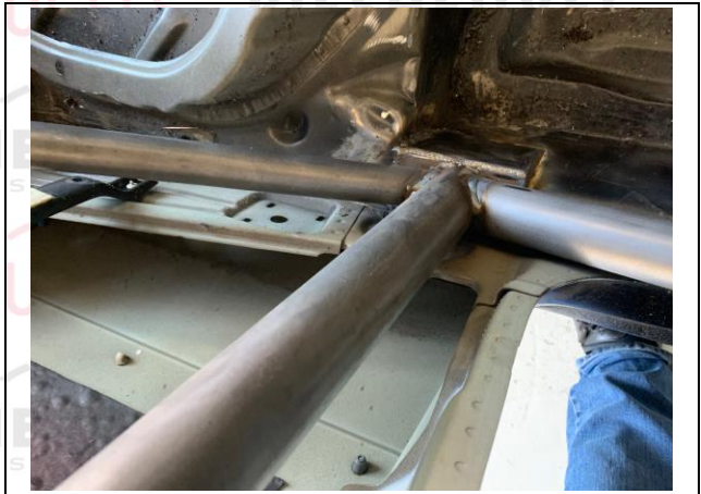
PHOTO 4 MAIN ROLLBAR TO FLOOR ATTACHMENT
